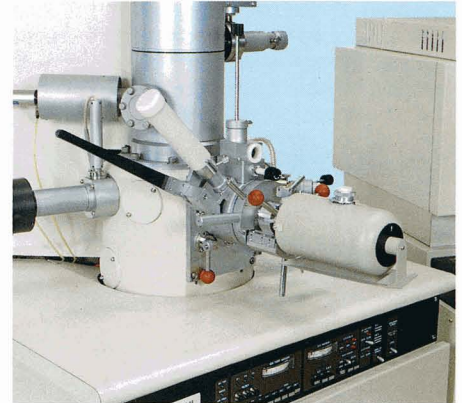
Cryogenic system mounted on the S-800
